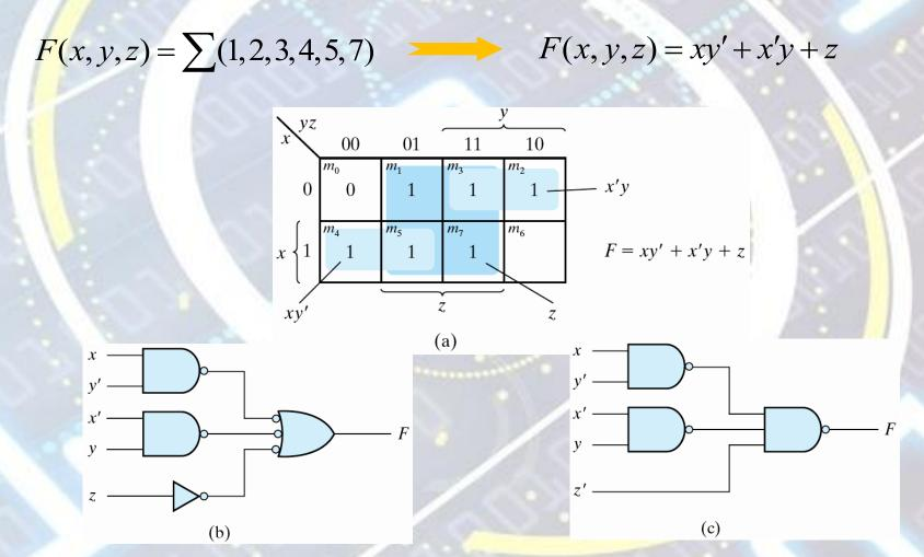
Figure 3.21 Solution to Example 3-10
