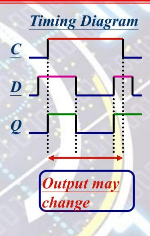
Controlled latches are level-triggered
