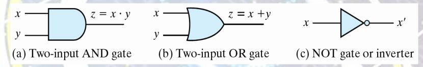
Fig. 1.4 Symbols for digital logic circuits
