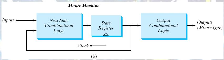
Fig. 5.21 Block diagram of Mealy and Moore state machine
