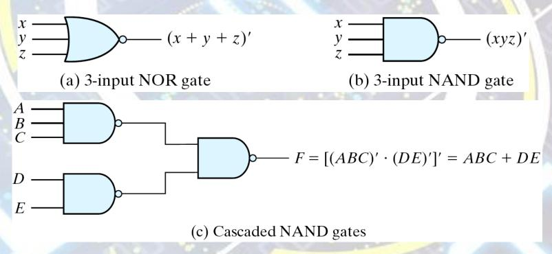
Figure 2.7 Multiple-input and cascated NOR and NAND gates
