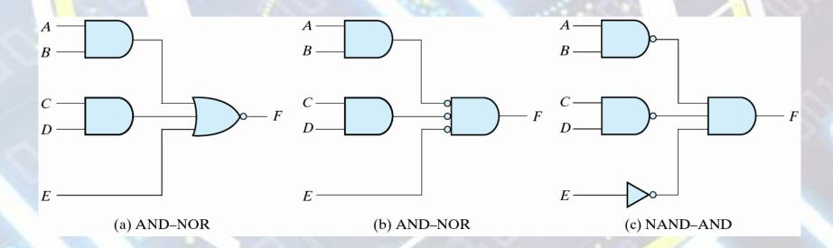
Figure 3.29 AND-OR-INVERT circuits, F = (AB + CD + E)'
