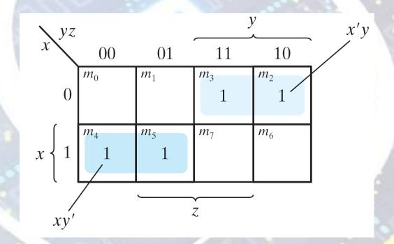
Figure 3.4 Map for Example 3.1,  $F(x, y, z) = \Sigma(2, 3, 4, 5) = x'y + xy'$
