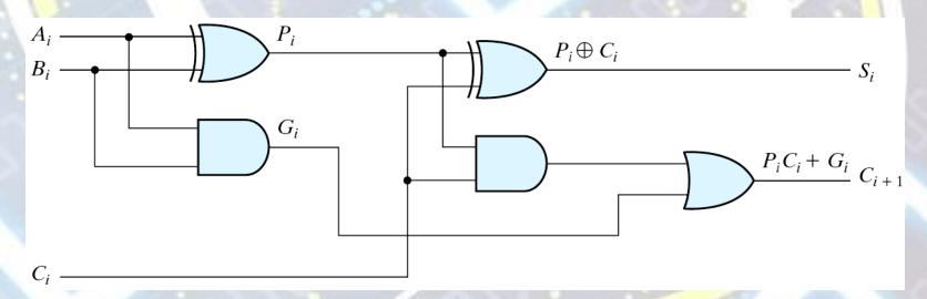
Figure 4.10 Full Adder with P and G Shown
