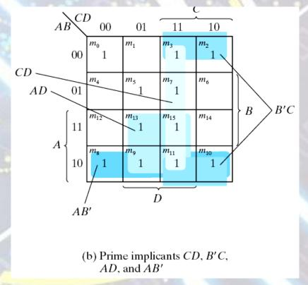
Figure 3.11 Simplification Using Prime Implicants
