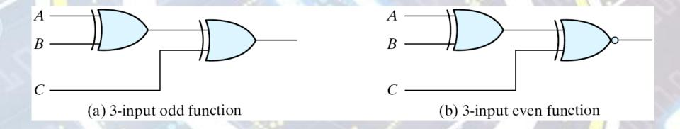
Figure 3.34 Logic Diagram of Odd and Even Functions
