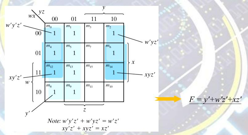
Figure 3.9 Map for Example 3-5;  $F(w, x, y, z) = \Sigma(0, 1, 2, 4, 5, 6, 8, 9, 12, 13, 14) = y' + w'z' + xz'$
