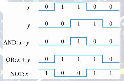
Fig. 1.5 Input-Output signals for gates
