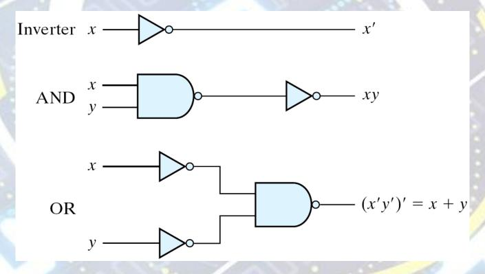
Figure 3.18 Logic Operations with NAND Gates
