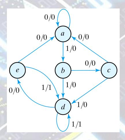
Fig. 5.26 Reduced State diagram
