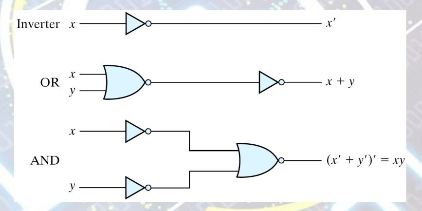
Figure 3.24 Logic Operation with NOR Gates
