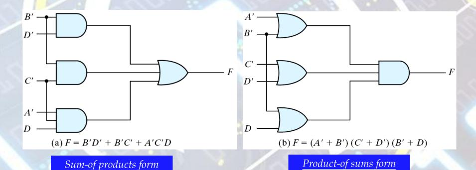
Figure 3.15 Gate Implementation of the Function of Example 3.8
