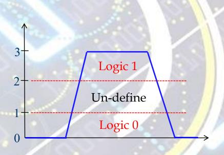
Figure 1.3 Example of binary signals
