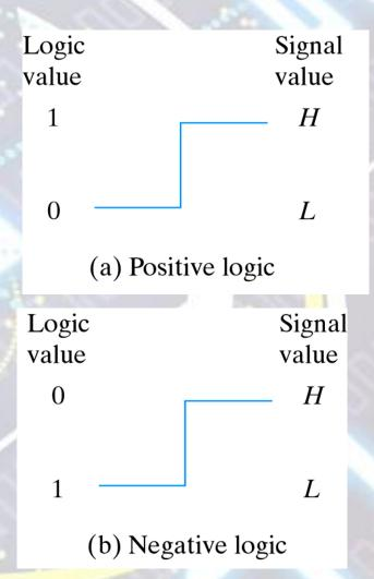
Figure 2.9 Signal assignment and logic polarity
