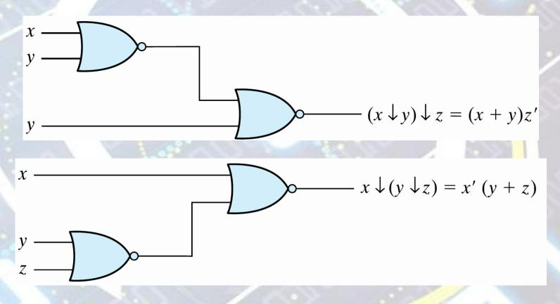
Figure 2.6 Demonstrating the nonassociativity of the NOR operator;  $(x \downarrow y) \downarrow z \neq x \downarrow (y \downarrow z)$
