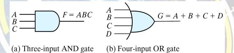
Fig. 1.6 Gates with multiple inputs
