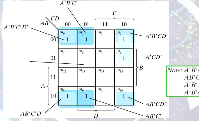
Note: A'B'C'D' + A'B'CD' = A'B'D' AB'C'D' + AB'CD' = AB'D' A'B'D' + AB'D' = B'D'A'B'C' + AB'C' = B'C'
